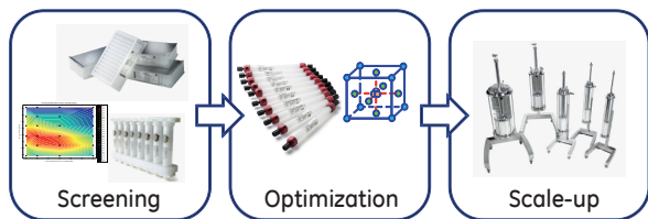
Fig 6. The recommended workflow is described in the figure. It starts with screening of conditions in high throughput formats, followed by optimization, preferably by applying Design of Experiments (DoE), in small columns and finally scale-up to large columns.
