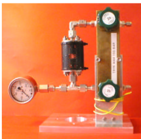
Photo showing the sapphire tube cell.
