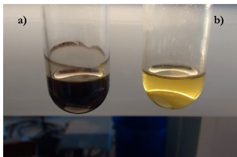
Difference between reactions running with a) 10% of ligand and b) 15%. The first one show catalyst decomposition responsible for the black color, while the second is clear.
